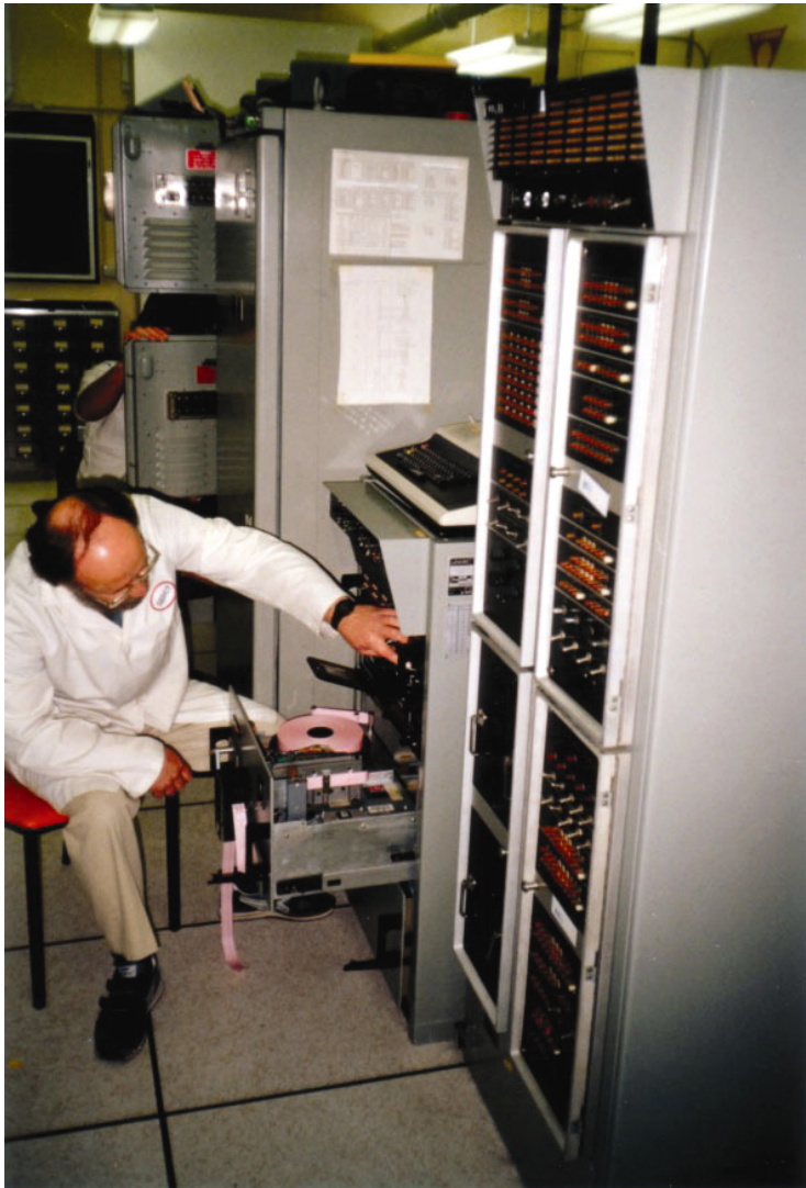
Pat Lynch working on the Mk95 IO console of the Mk152 computer in the DDG equipment room
