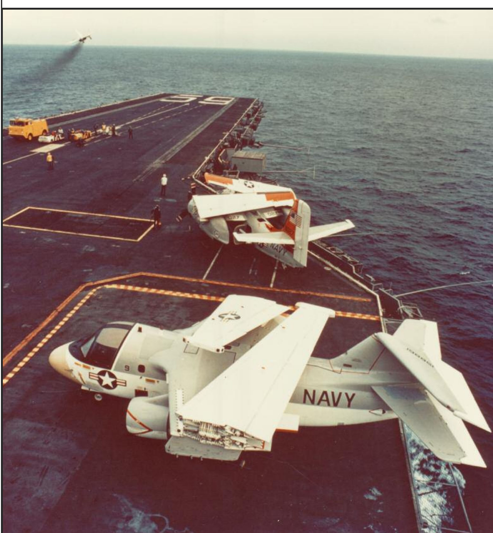
Below left: An image of an S-3 airplane (front) with its wings folded, sitting atop an aircraft carrier. Below right: The "T" shaped UNIVAC 1832 airborne computer installed in the rear of an S-3A airplane.
