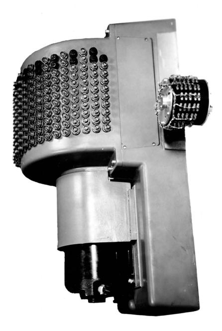
Magnetic Storage Drums - Incremental Computer and Univac Scientific
