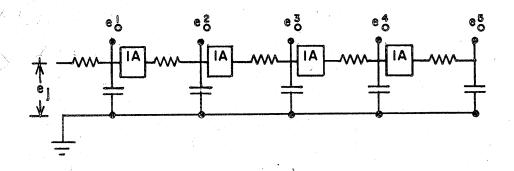
This program was run numerically on a simulation routine in an 1103 large scale computer to obtain the frequency response of the system and the five outputs agreed in amplitude and phase shift with that expected from filter theory.
