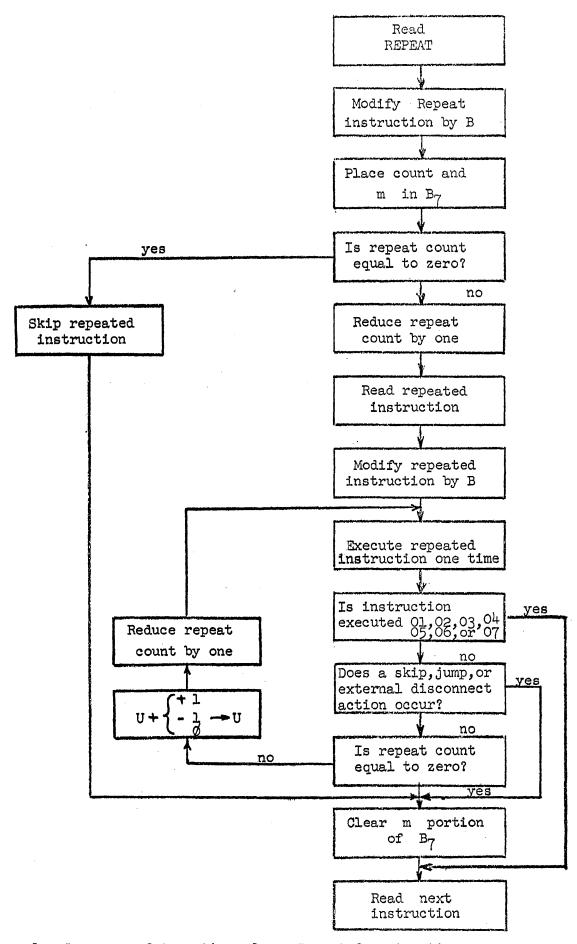
Figure 2 - Sequence of Operations for a Repeated Instruction
