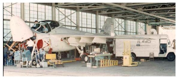
ILAAS002: SSMD engineers at work on the A6. The equipment including the Univac-supplied computers (1818), Fault Sensing Units (FSU) and Flight Test Memories (FTM) were housed in the nose of the aircraft. The FTMs were ground support equipment and were never intended to fly, but SSMD flew them, and they performed as well as the environmentally tested computers.
