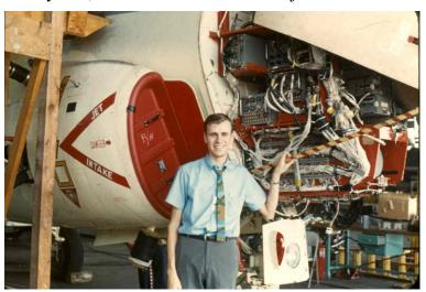
ILAAS005: Bob Wochinger, SSMD software engineer, probably entering a navigation software patch into the Univac Flight Test Memory (FTM) via its control panel (black). Above the FTM control panel is a Univac ILAAS computer Control Panel (gray) and connecting cables and to their right are two control panel isolation networks for connecting to the computer during ground support.
