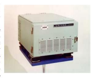
faster than the UYK-20 and, given the fact that the CPUs micro programmable controller also served as the I/O controller, under high I/O bandwidth conditions brought the processor to a stop. The 1616 design used in the UYK-15 had an independent I/O Controller and in most installations had an independent port into a four-port memory.
