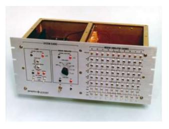
drivers and the associated hardware interfaces were working. It used a wire-wrapped circuit module for the control circuitry which was made up of standard 5400 TTL IC's.
