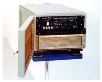
I had done a four-port memory front end design for Project Outboard which was primed by Sanders Associates. A second half-sized cabinet was added below the unit pictured and the memory buses were daisy-chained (a tough trick) from the top cabinet to the expansion cabinet. The Sanders RF signal processing system used the fourth port. Virtually all of the production UYK-15 installations used the expansion cabinet as that provided a total of 64K x 16-bit words and the
