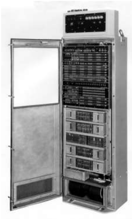
Picture 4b – left: EDM with front door open showing the relationship of the 32K-Word Core memory unit to the Maintenance Panel.
