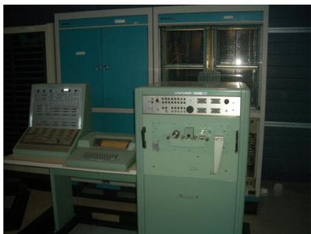
The maintenance panel setting on the 1232 desk adjacent to the keyboard/printer is for the UNIVAC Type 1230 MTC computer, which was at Sunnyvale CA for almost three decades.
