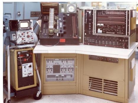
In today's vernacular, we have flash drives, USB sticks, RAM, hard drives, etc. None of these technologies has the radiation resistance levels that were required for the Minuteman computers – met by the use of plated wire memory instead of the more susceptible core memory of that generation. Submitted by LABenson
