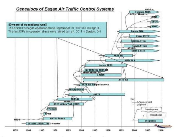
The Input Output Processor (IOP) of ARTS III is a 30-bit machine using the same basic Instruction Set Architecture (ISA) as the Naval Tactical Data Systems of the 60s-80s. The lead IOP logic designer was John Bonnes, BEE 1965 - University of Minnesota.
