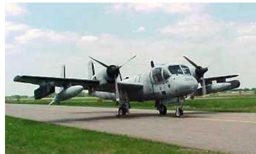
Grumman RV1C had Sensor Pods and Gas Tanks under the Wings
