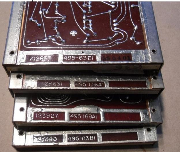
These are 4.5" x 6", with ~33 pin connectors. The P/Numbers at the left are most likely Assembly Part Numbers, stamped at the right are manufactured dates, i.e. 58 0401. What is the center 495-... number?
