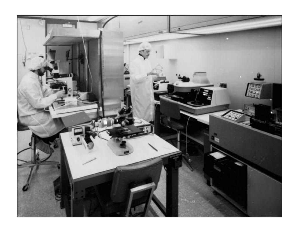
Above: Sperry employees working in a clean-room setting. Making semiconductors requires a tightly controlled environment. From the early 1950s up to the 1990s UNIVAC maintained a state-of-the-art failure analysis laboratory. If its suppliers' parts were defective, they were asked to take corrective action. Semiconductors
