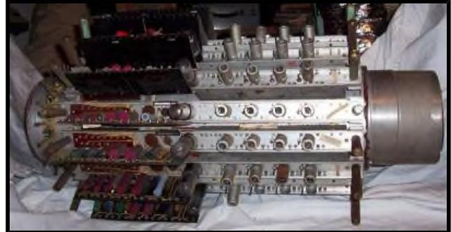
The seven long tanks of UNIVAC I were harnessed together in an electronic circuit called a whiffletree, which is a word not often used today and it somewhat fascinated me that it was used in describing the mercury memory linkage of UNIVAC I. You can see what that whiffletree looks like in a diagram near the end of this page. It could be valuable information if you ever come across a long tank.
