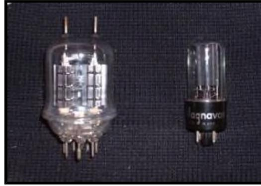
**Type of tubes used in UNIVAC I systems.**
