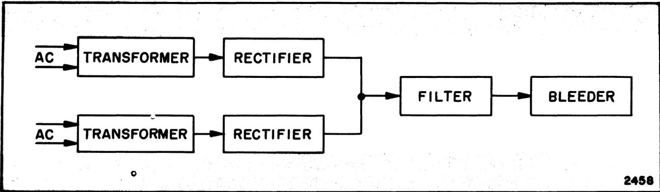
Figure 1-24. Power-Supply Rectifier Circuits
