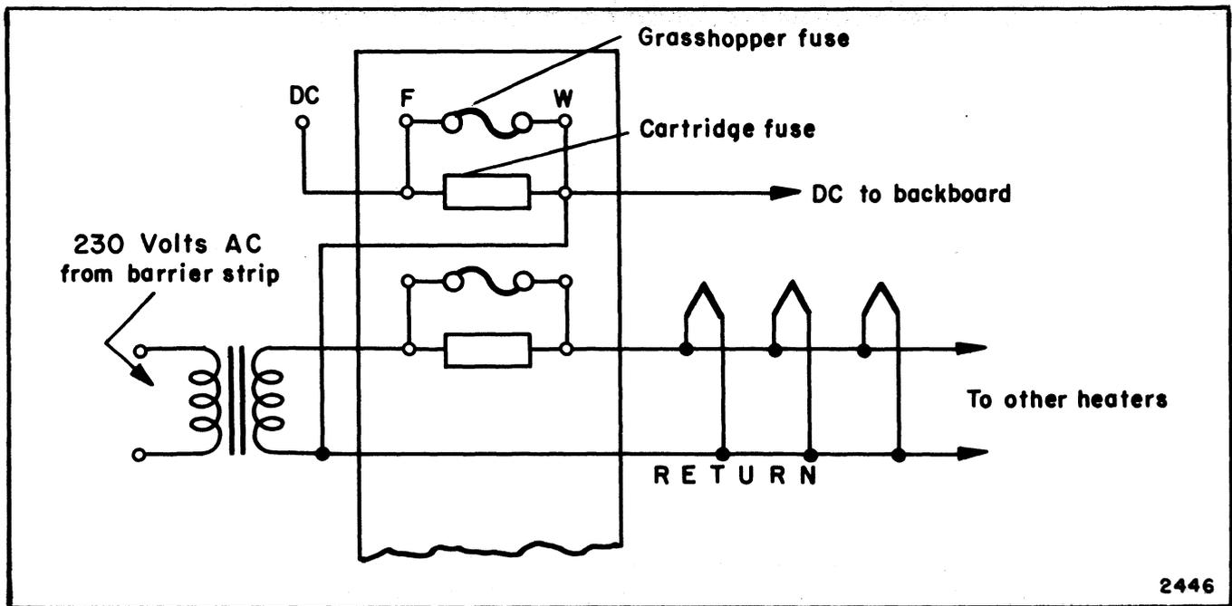
Figure 1-12. Minimizing of Heater-to-Cathode Arcing
