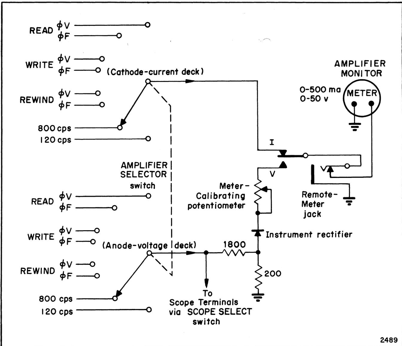
Figure 2-25. Amplifier Monitor Section, BC Corner Box
