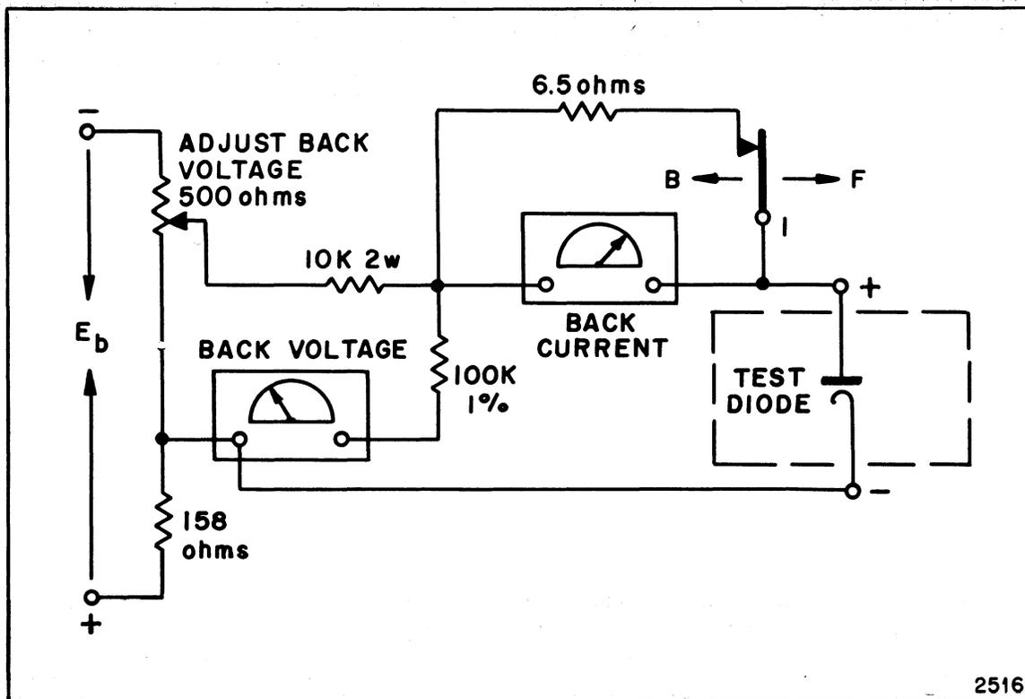
Figure 3-9. Diode Tester for Back-Current Check
