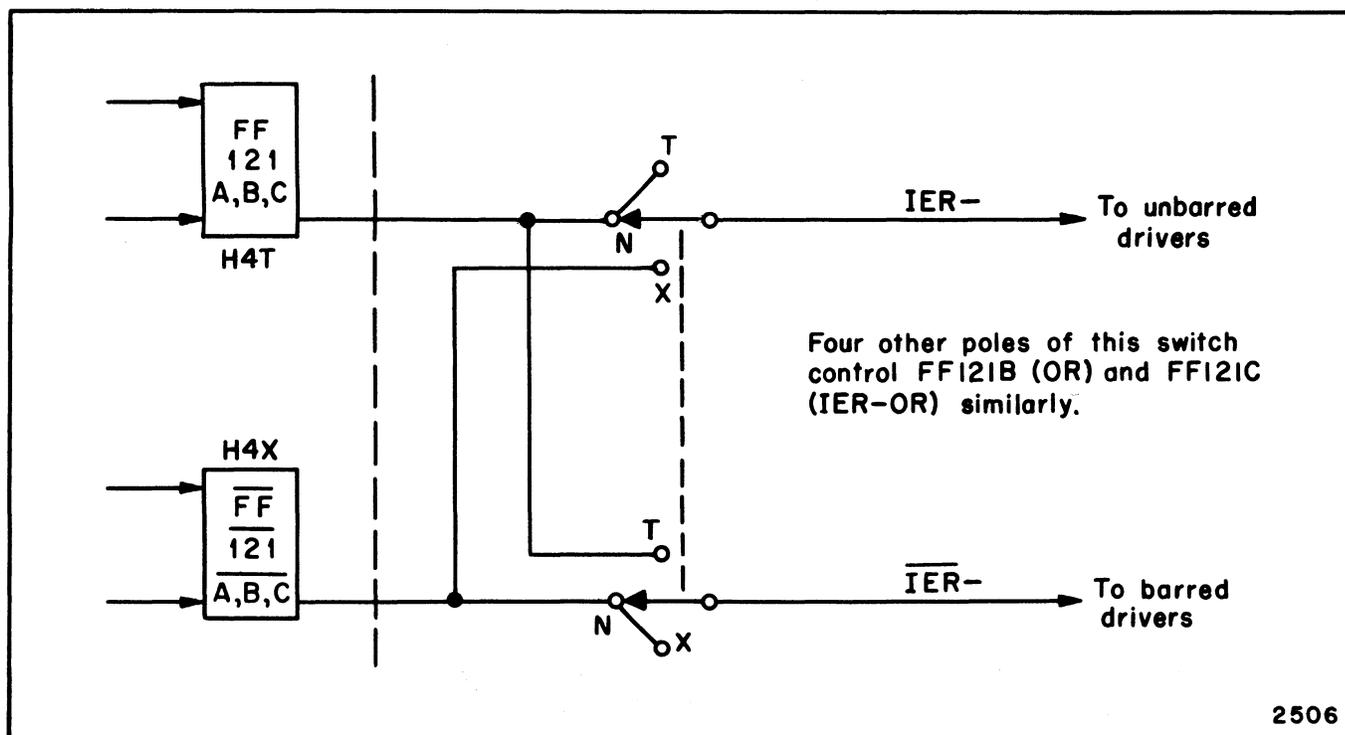
Figure 2-43. IER/OR Test Switch on H4X Backboard
