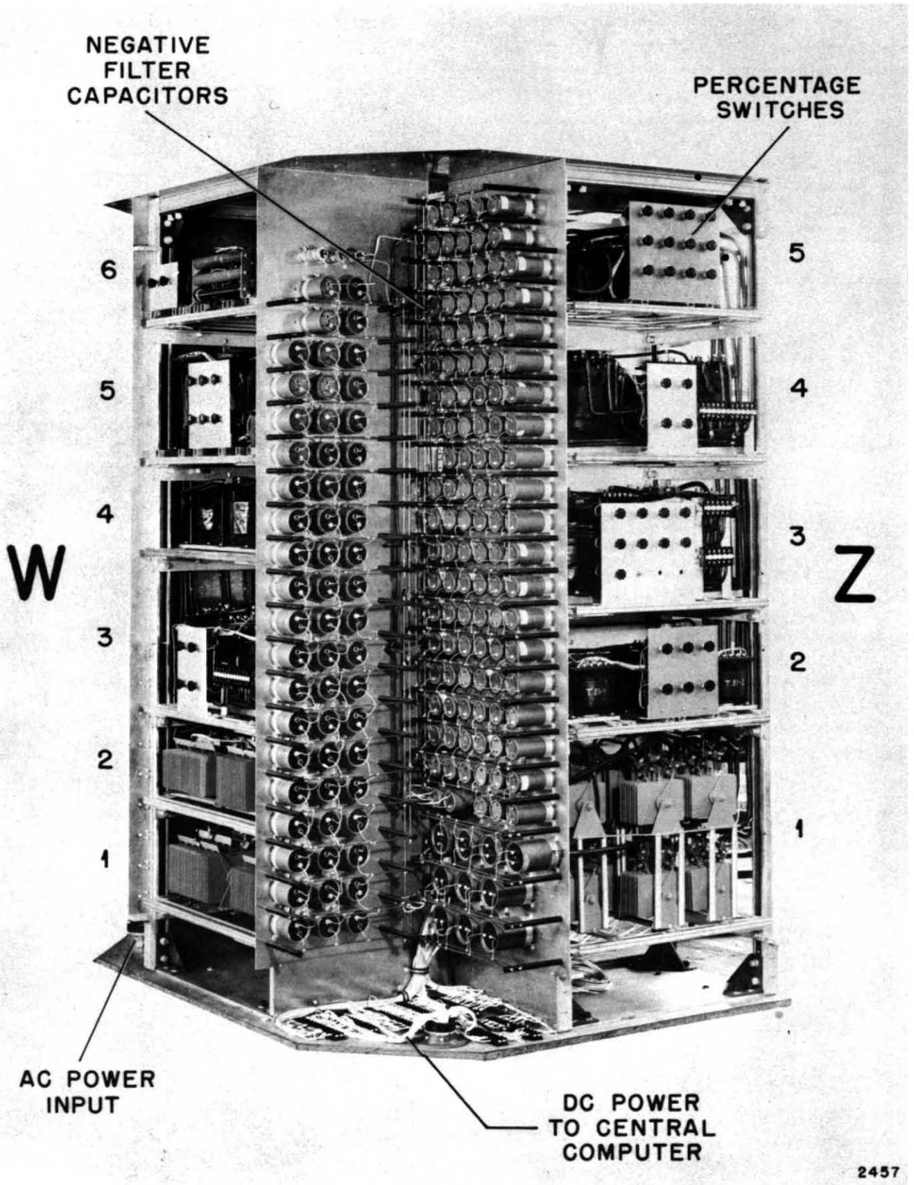
Figure 1-23. Power Supply, Casework Removed
