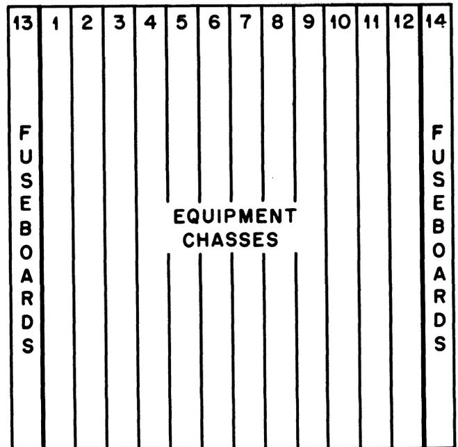
**Figure 1-3. Standard Section Layout**
