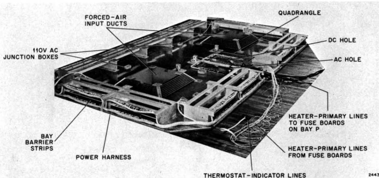
Figure 1-9. Sub-Floor Assembly
