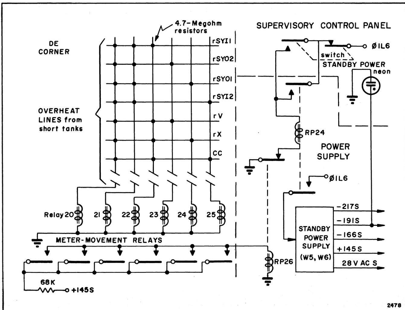
Figure 2-14. Short-Tank Overheat System, Schematic
