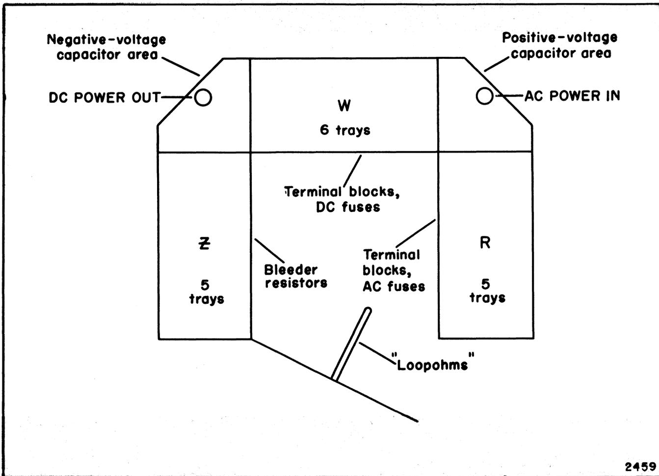
Figure 1-25. Power-Supply Layout
