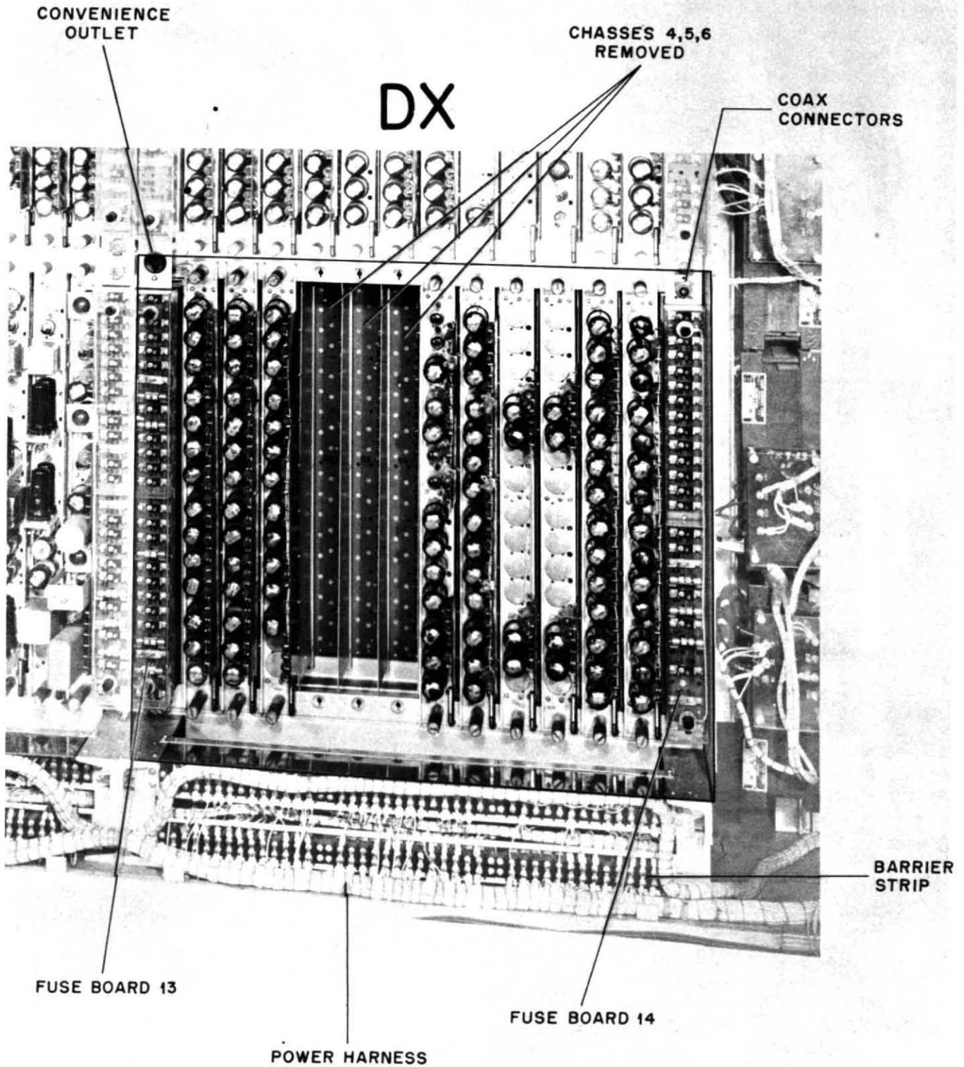
Figure 1-6. Section Detail
