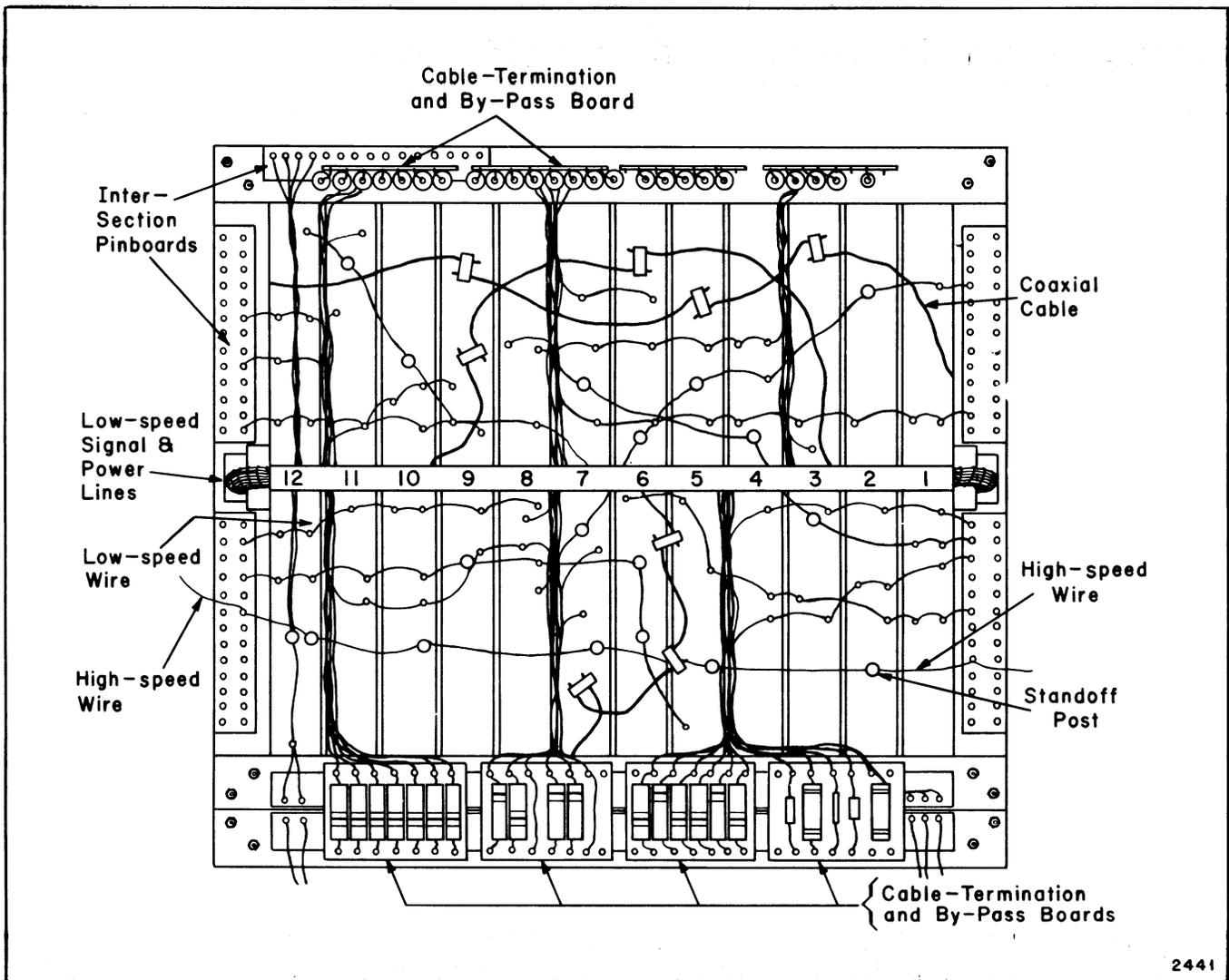
Figure 1-7. Section Detail, Rear View
