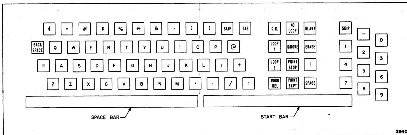
**Figure 5-2. Supervisory Control Panel Keyboard**
