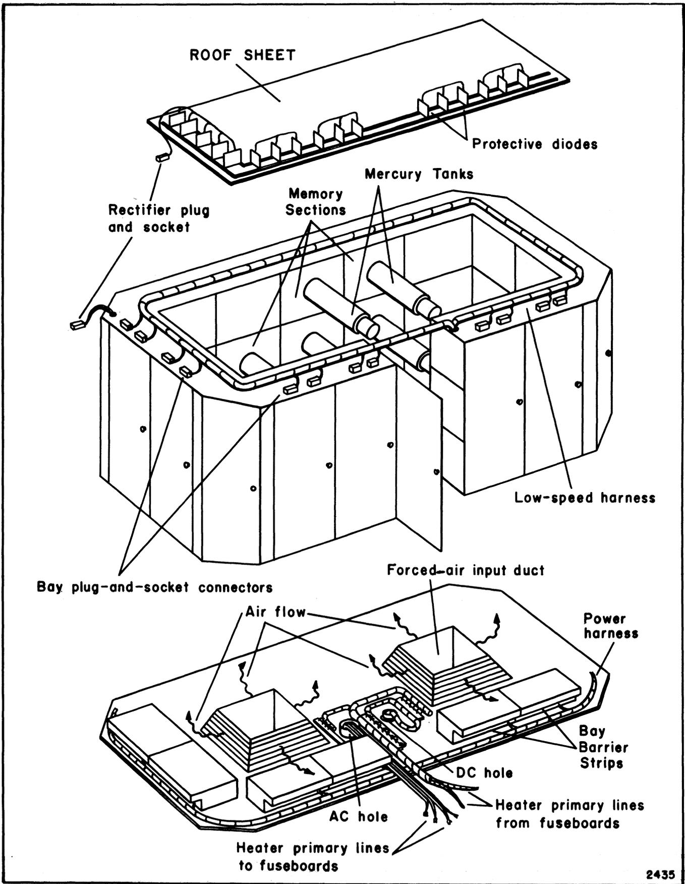
Figure 1-1. Exploded View of Univac I Central Computer
