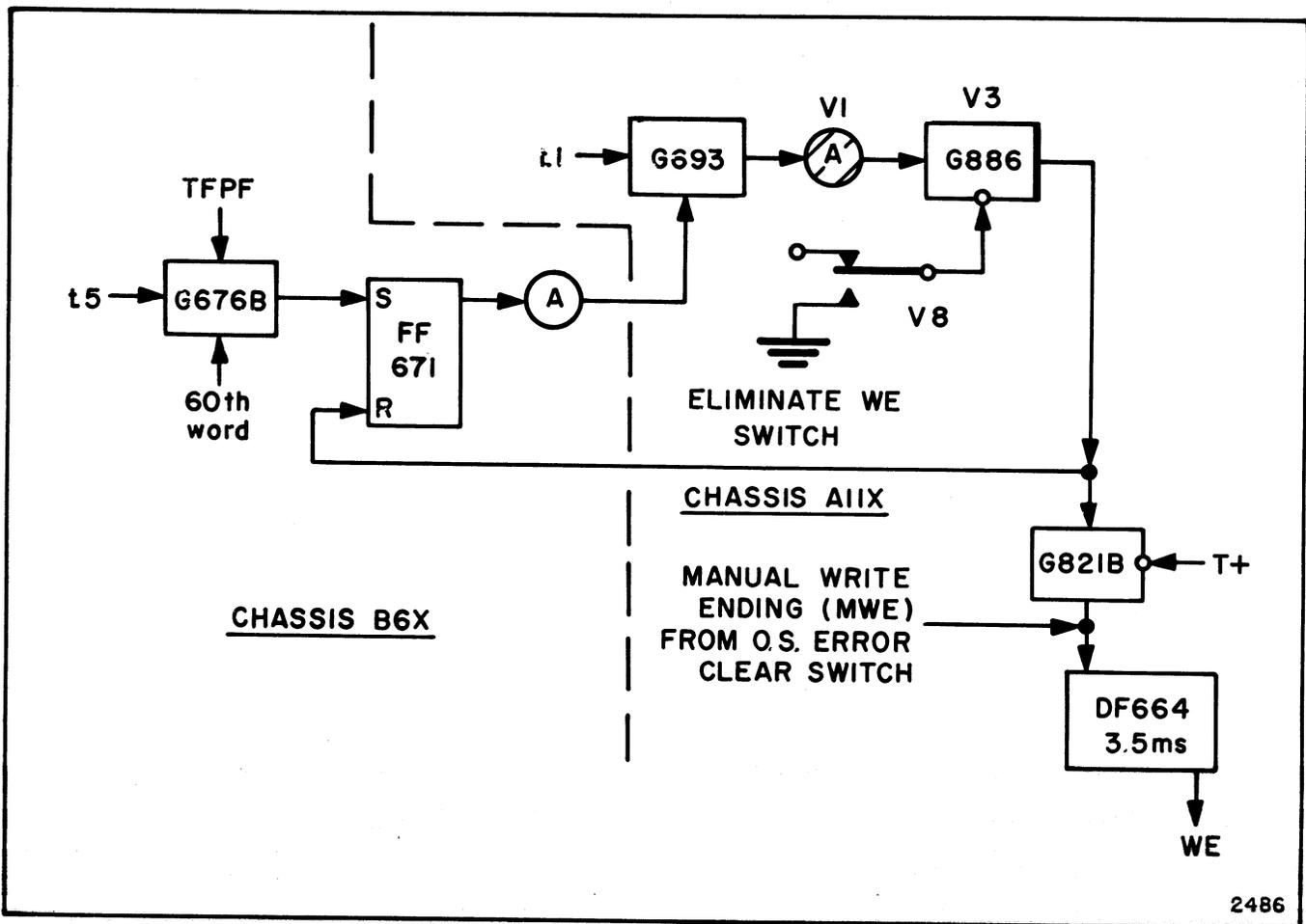
Figure 2-22. Write-Ending Circuit
