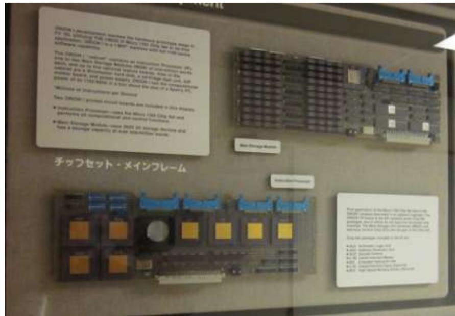
(MSUC) and Interface Controller Chip (ICC) are not part of the Chip-Set. Chip-Set packages included in the IP are: ALU- Arithmetic Logic Unit, AGU- Address Generator Unit, DCD- Decode Control, CIM- Cache Interface Master, EIS- Extended Instruction Set, CIS- Cache Interface Slave(Optional), and M/D- High Speed Multiply /Divide (Optional).
