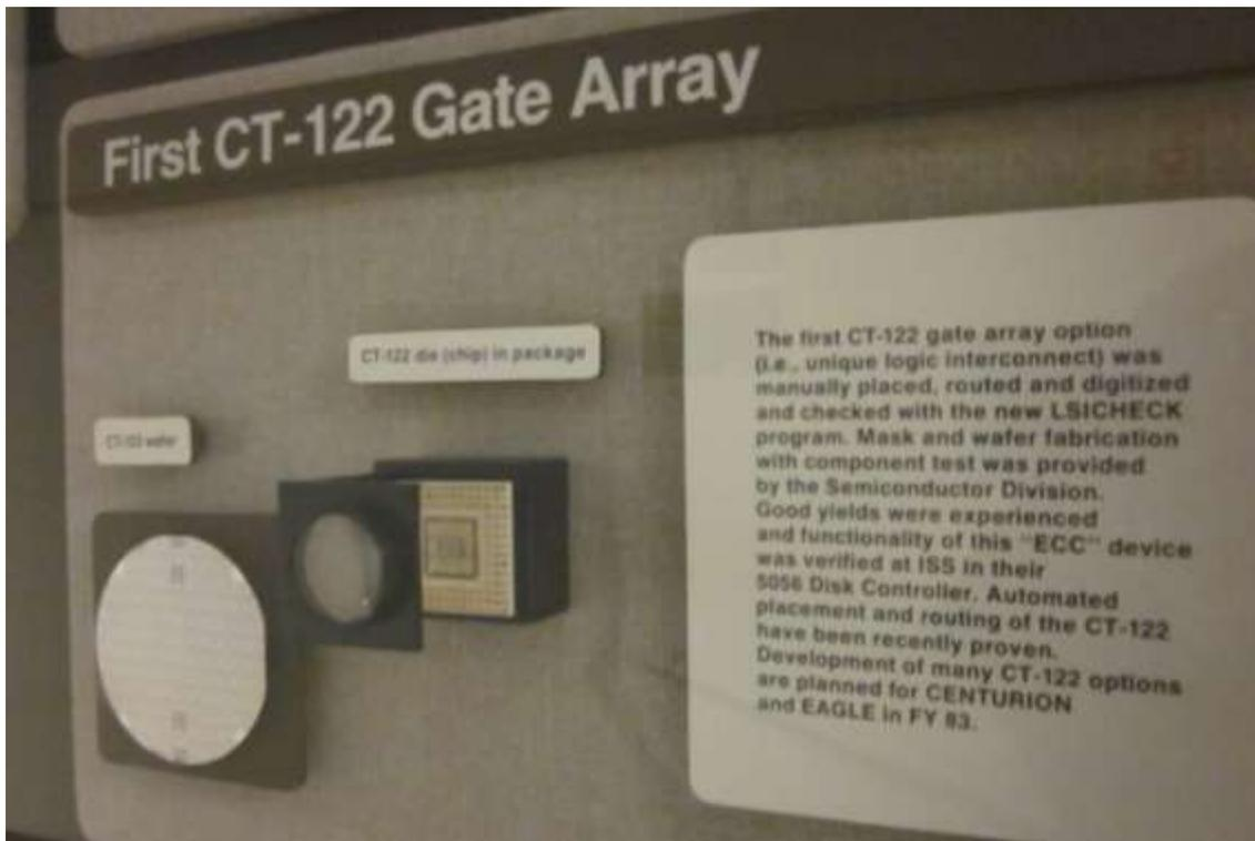
interconnect) was manually placed, routed and digitized and checked with the new LSICHECK program. Mask and wafer fabrication with component test was provided by the Semiconductor Division. Good yields were experienced and functionality of this "ECC" device was verified at ISS in their 5056 Disk Controller. Automated placement and routing of the CT-122 have been recently proven. Developments of many CT-122 options are planned for CENTURION and EAGLE in FY'83.
