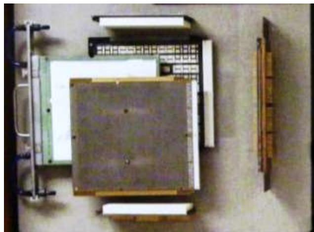
**FIRST SAM DELIVERY FOR 1100/80** - The Scientific Accelerator Module for the 1100/80 is a special capability for scientific users and a market expansion product for Sperry Univac. Built from the first gate array LSI logic chips designed in Roseville. The technology is a leader in the design capability needed for the S-80 and Chaparral. *Card assembly with 14 LSI chips.*
