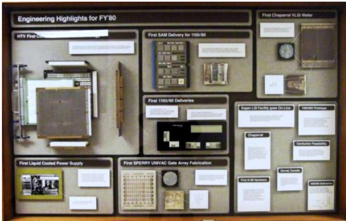
**HTV FIRST CONSTRUCTION OF S-80 TECHNOLOGY** - The Hardware Test Vehicle (HTV) constructed from S-80's new sub nanosecond emitter coupled logic (SNECL) is now under test, cooled by water and highly compact in construction. *The basic assembly is a cooling plate sandwiched between two circuit boards with wire-wrap connector.* Twenty-six of these assemblies will comprise the total S-80 instruction processor.
