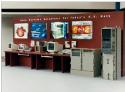
Left: A picture of the AN/UYK-43 (far right) and AN/UYK-44 (on table in middle) and other associated company products. The UYK-43's various components were designed to work in concert with one another to provide a real-time response. In many situations, the seconds that this buys is critical.
