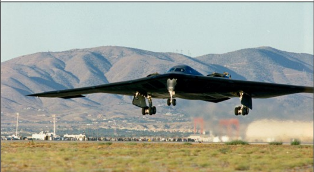
Below: An image of a B-2 Bomber taking off. The aircraft has a crew of two and can carry up to 16 2,400 lb nuclear bombs. It can fly at 50,000 feet and has a range of over 6,000 miles on one tank of fuel.
