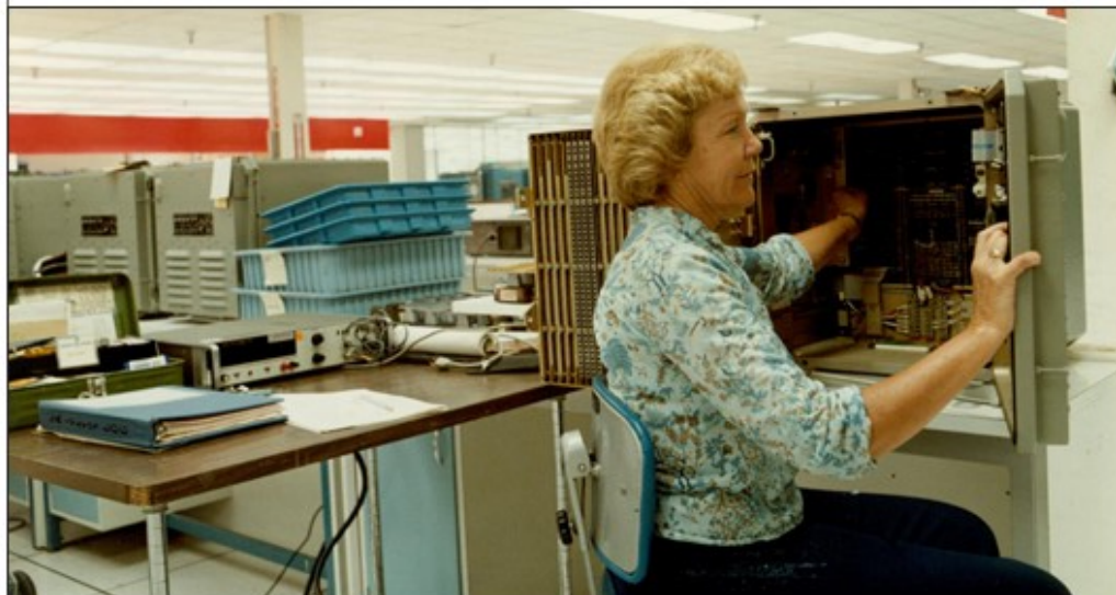
Below: A Sperry UNIVAC employee assembling a AN/UYK-20 minicomputer at the company's Clearwater, Florida, plant. While the units were designed in Eagan, they were assembled in Florida.
