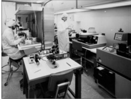
Above: Sperry employees working in a clean-room setting. Making semiconductors requires a tightly controlled environment. From the early 1950s up to the 1990s UNIVAC maintained a state-of-the-art failure analysis laboratory. If its suppliers' parts were defective, they were asked to take corrective action. Semiconductors finally became more reliable in the 1980s.
