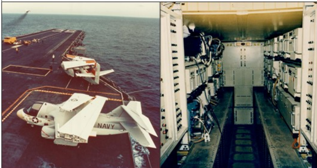
Below left: An image of an S-3 airplane (front) with its wings folded, sitting atop an aircraft carrier. Below right: The "T" shaped UNIVAC 1832 airborne computer installed in the rear of an S-3A airplane.
