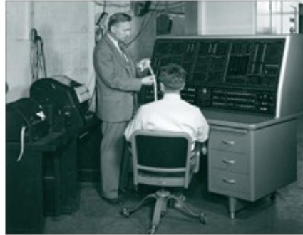
Above: ERA engineer Jack Hill inspecting the tape from an early company computer. The first "software" was coded this way and was later replaced by punch cards.
