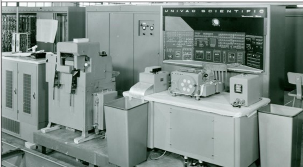
Below: A continuation of their 1100 computer series, UNIVAC rebranded an upgraded 1103 computer as the "UNIVAC Scientific." Its commercial successors, the 2200 series from Unisys, continued into the 1990s.
