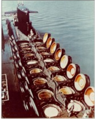
Above: A picture of the Lafayette Class USS Sam Rayburn with all of its hatches open. Decommissioned in 1989, it had a capacity of 16 intercontinental ballistic missiles (ICBMs) and 21 torpedoes.
