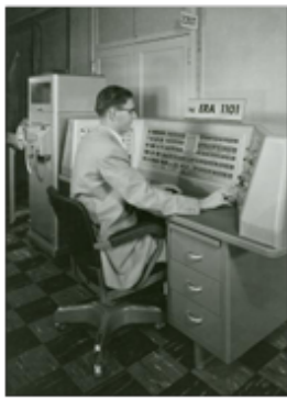
Left: Engineer Earl Joseph programming ERA's first true computer: the 1101. Only two units were ever built. Because ATLAS was the 13th item on ERA's first Navy contract, the commercial version was named 1101 which is binary for 13. Its successor, the 1103, was an immediate commercial success upon completion in 1953; 20 units were sold in the following years.
