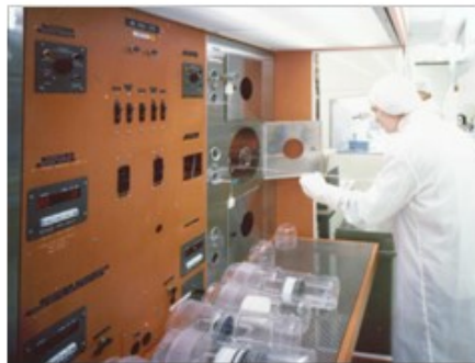
Above: Sperry employees working in a clean-room setting. Making semiconductors requires a tightly controlled environment. From the early 1950s up to the 1990s UNIVAC maintained a state-of-the-art failure analysis laboratory. If its suppliers' parts were defective, they were asked to take corrective action. Semiconductors finally became more reliable in the 1980s.
