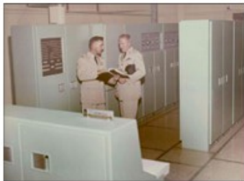
Left: A picture of the Athena II Computer - the successor to the first Athena. Athena was the first Univac-produced computer to use transistors. A transistor is a device that helps control the flow of electricity in a machine. Prior to transistors, engineers had used vacuum tubes inside of computers which frequently caused overheating.
