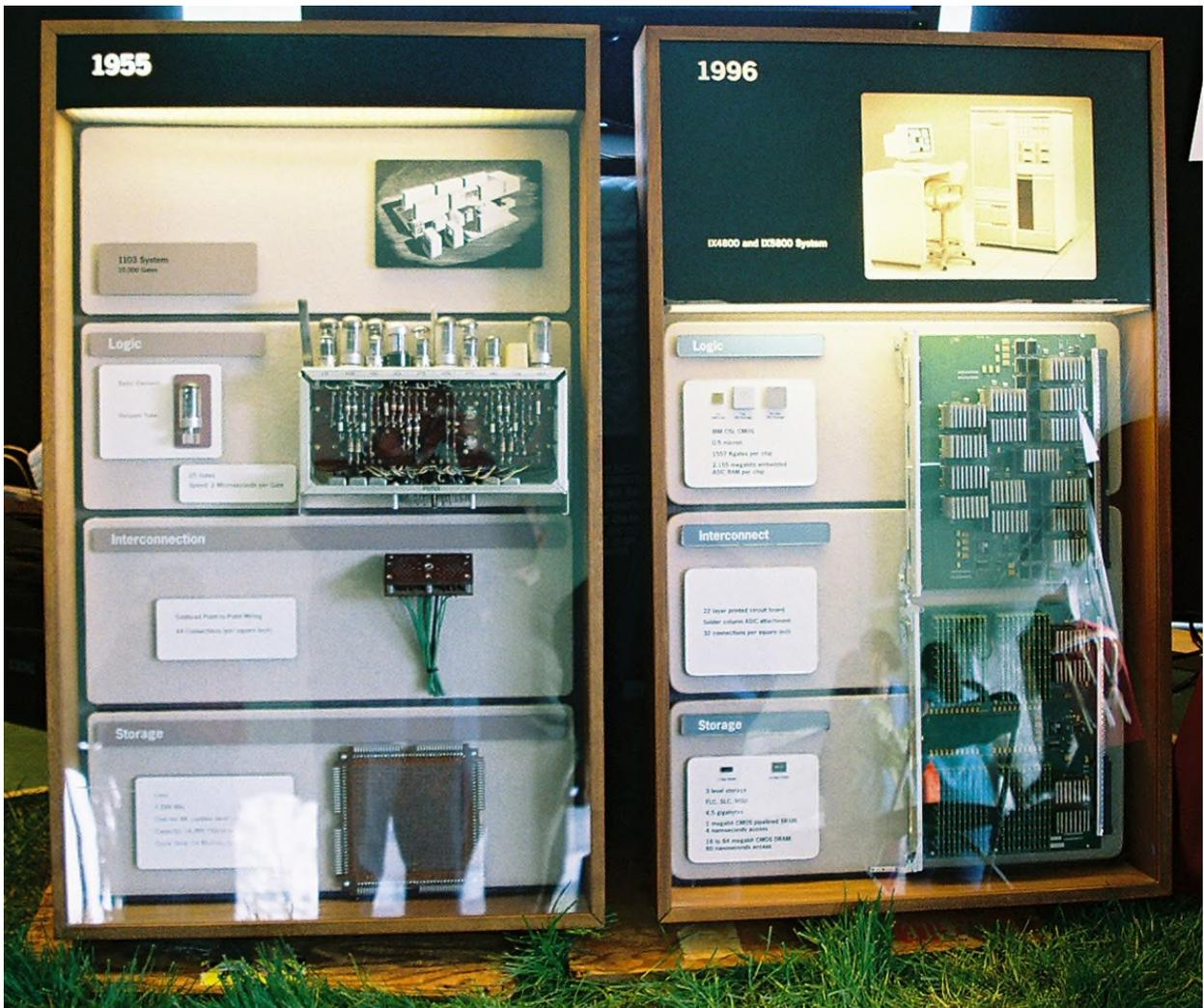
Picture 4 - UNISYS also provided a couple displays from their Roseville Plant 4 history wall – these show 1955 versus 1996 circuit and memory technologies.
