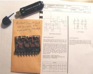
up the 1958 NTDS CP-642A unit computer. The 6"x 8.5" sheet of paper at the right of the snapshot shows the general schematic and logic diagram of the cards 1960's spare parts replacement design including four PNP transistors [gates].
