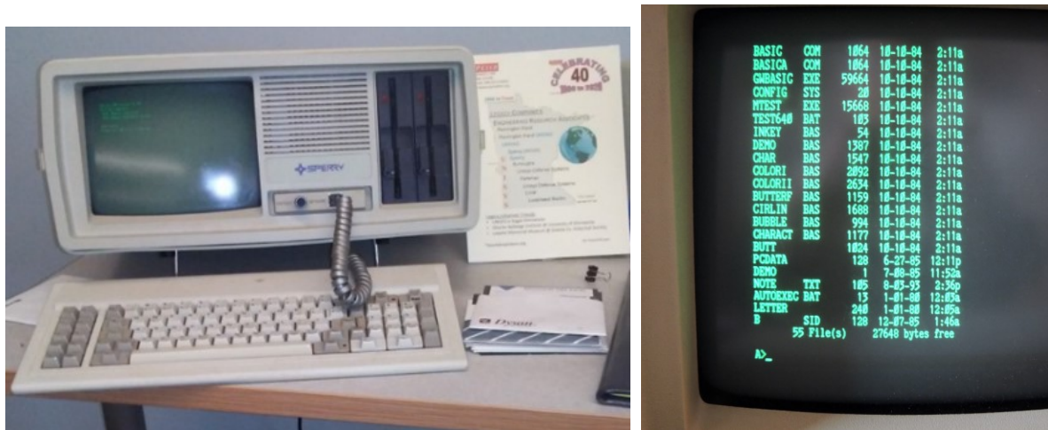
Figure 7. This suitcase computer from the 60's used 5.25" floppies and a Disk Operating System (DOS). The DOS Dir A: typed command yielded the disc contents. First in this list (right image) is BASIC.COM, software used to generate .EXE executable files from the .BAT input files, snapshots by LABenson.
