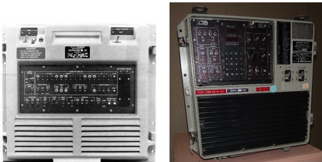
Figure 8. The AN/UYK-502 11 developed in the 70s had typical 16-bit register indicators, whereas the AN/UYK-44 12 in the 80s used a hexadecimal keypad and a small LED screen for internal register readouts, snapshots by Keith Myhre.
