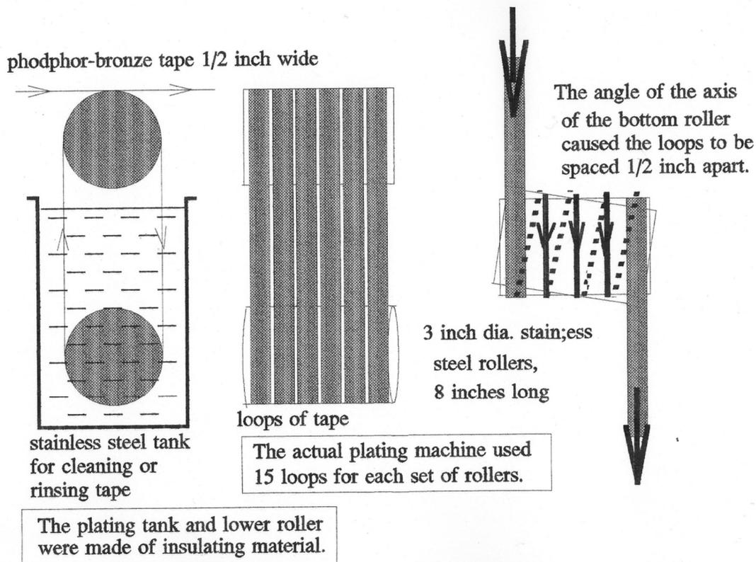
The tape was moved at a speed of around six inches per second [twelve for the second machine] by a motor that turned the top roller [or rollers] over the electroplating bath. The take up spool was turned by a motor with enough torque to just keep the spool turning. Also several roller stations before the plating bath were powered by motors controlled by sensors in order to prevent damage from excessive tension on the tape.
