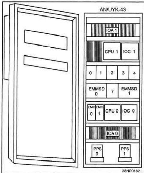
Illustrated at the left, one cabinet housed two CPUs, two IOCs, two IOA sets, dual power supplies, and numerous memory modules. An enhancement to the AN/UYK-43, the Open Systems Module (OSM), allows up to six Type 6U VME bus commercial off-the-shelf (COTS) cards to be installed in a UYK-43 enclosure.
