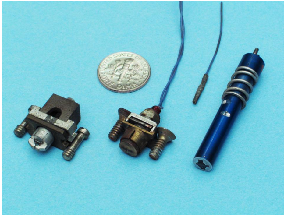
Photo B1 – Three types of heads. From left to right: Permanent magnet head with mounting screws, short head with twisted pair wires and with holder and mounting screws, one wire with taper pin termination, long head with spring.
