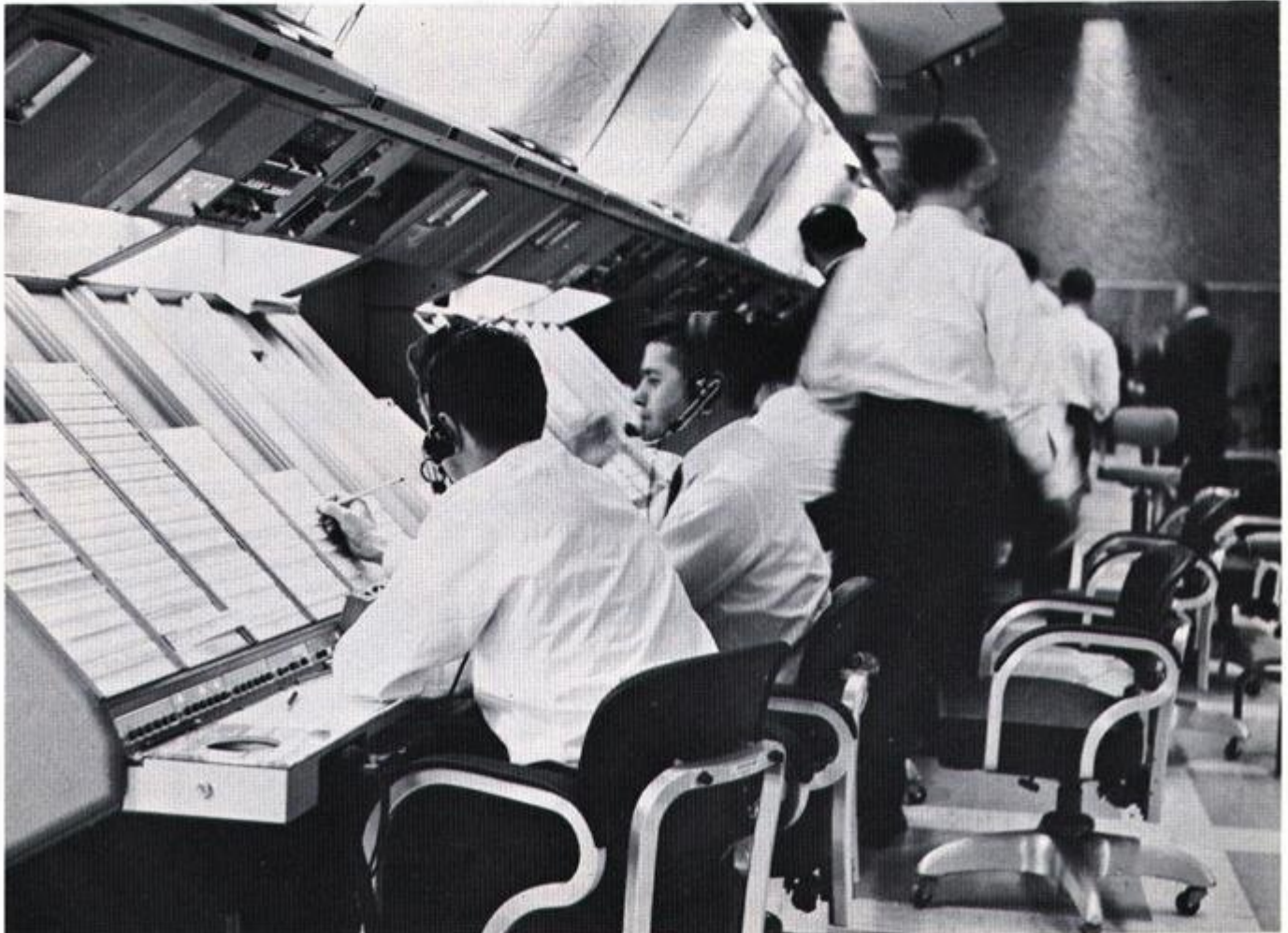
The men in this rank of controllers are receiving over telephones flight information for processing through the Univac System.
