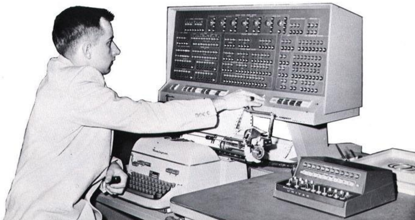
The control console is the nerve-center of the FAA Univac File-Computer installations. The inquiry typewriter is an important element in the system's input/output facilities. All photographs for this article were made at the Cleveland Control Center.
